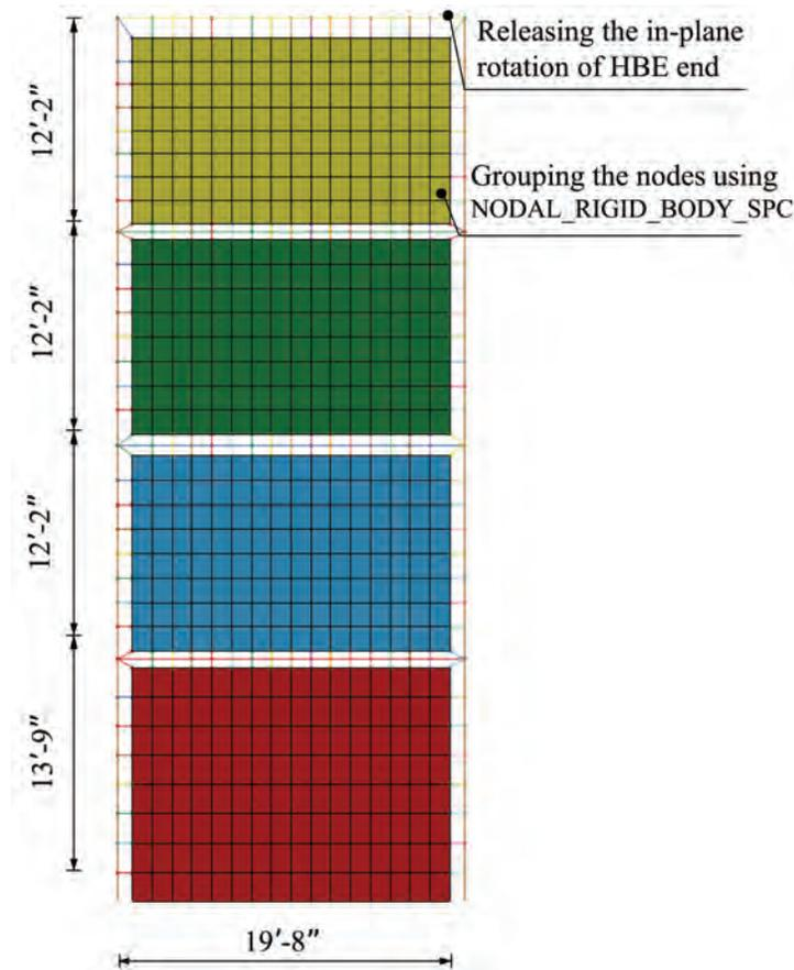
Fig. 1. Dimensions and constraints of four-story, limited-ductility SPSW.
