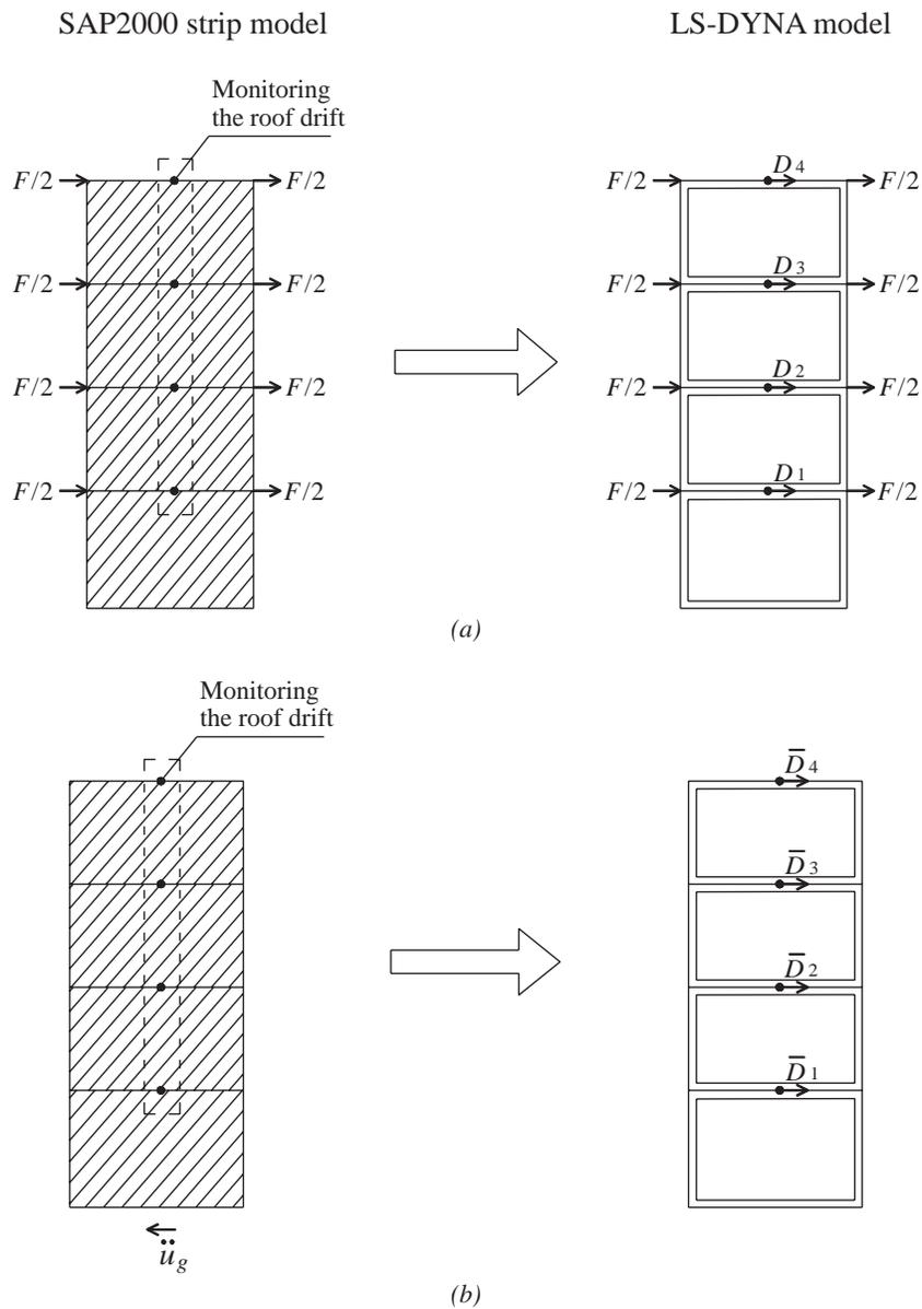
Fig. 5. Loading approaches for pushover analyses in SAP2000 and LS-DYNA: (a) uniform distribution of force; (b) inverted triangular force.  $D$  and  $\bar{D}$  refer to displacement histories from SAP2000 model subjected to uniform distribution of force (SP-40°-U and SP-45°-U) and inverted triangular force (SP-40°-T and SP-45°-T), respectively.
